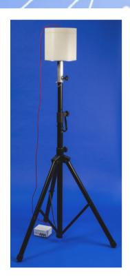
The NNS is the long-awaited, simple solution, for the routine field use of the well-known Bonner Sphere method. At the heart of the NNS are 7 moderating cylindrical shells, placed one inside the other, providing a lighter-weight compact instrument for neutron field characterization.
